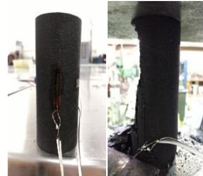
Intact Sample Failed Sample
