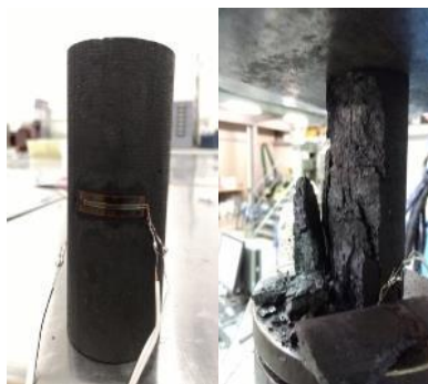
Intact Sample Failed Sample
