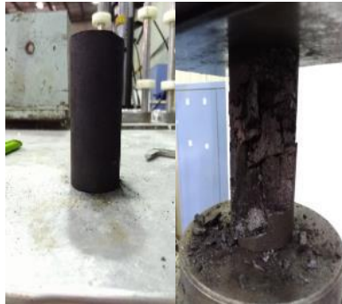
Intact Sample Failed Sample
