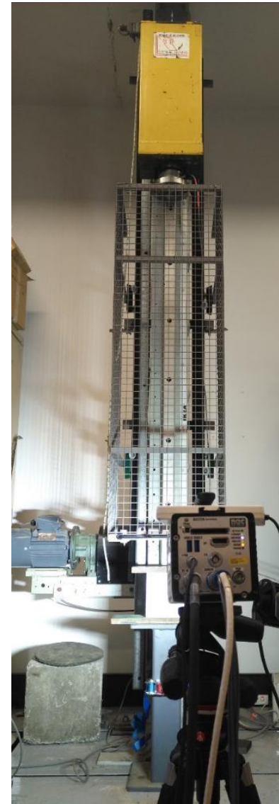
Drop hammer test system
