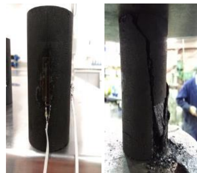
Intact Sample Failed Sample
