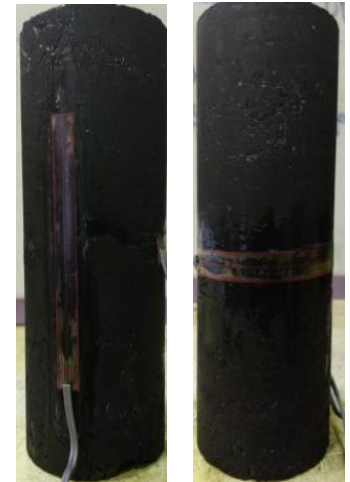
Coal Sample with Strain Gauges
